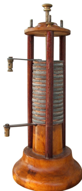
Fig. 2: Voltaic pile – source of constant DC voltage 3
